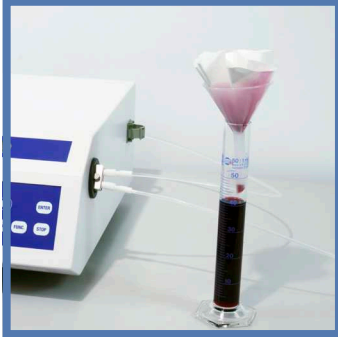
Filtration and degassing
