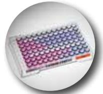
**The YeastOne plate's easy set up procedure eliminates the time-consuming macrobroth dilution method.**
